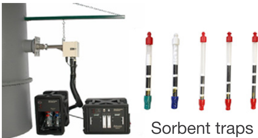
Figure 5: Sorbent traps and analyzer
