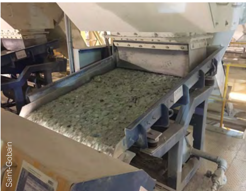
Figure 76: Glass being recycled into cullet
