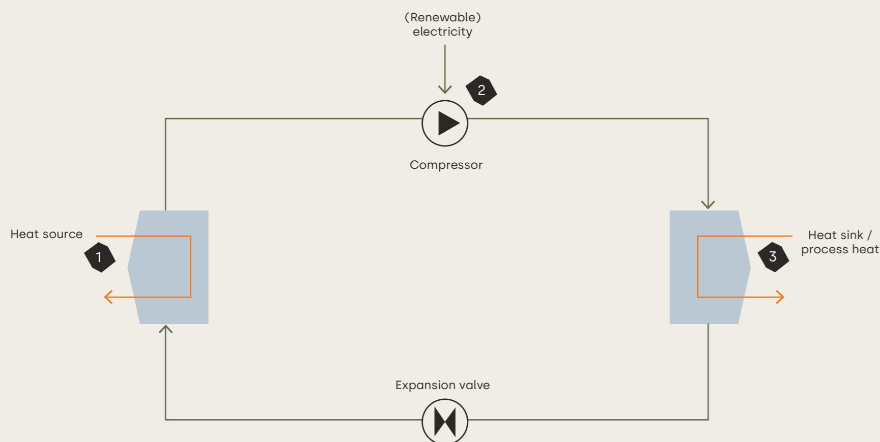
Figure 1: Simple diagram of a mechanical heat pump
