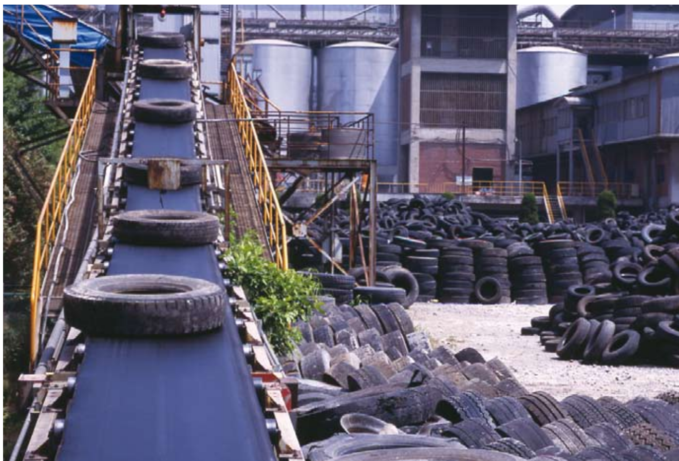
Tires sent for co-processing in a cement plant where both fuel value and materials are recovered
