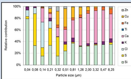
Figure 5a. PIXE analysis of airborne TWP (Michelin Pilot Primacy shown)
